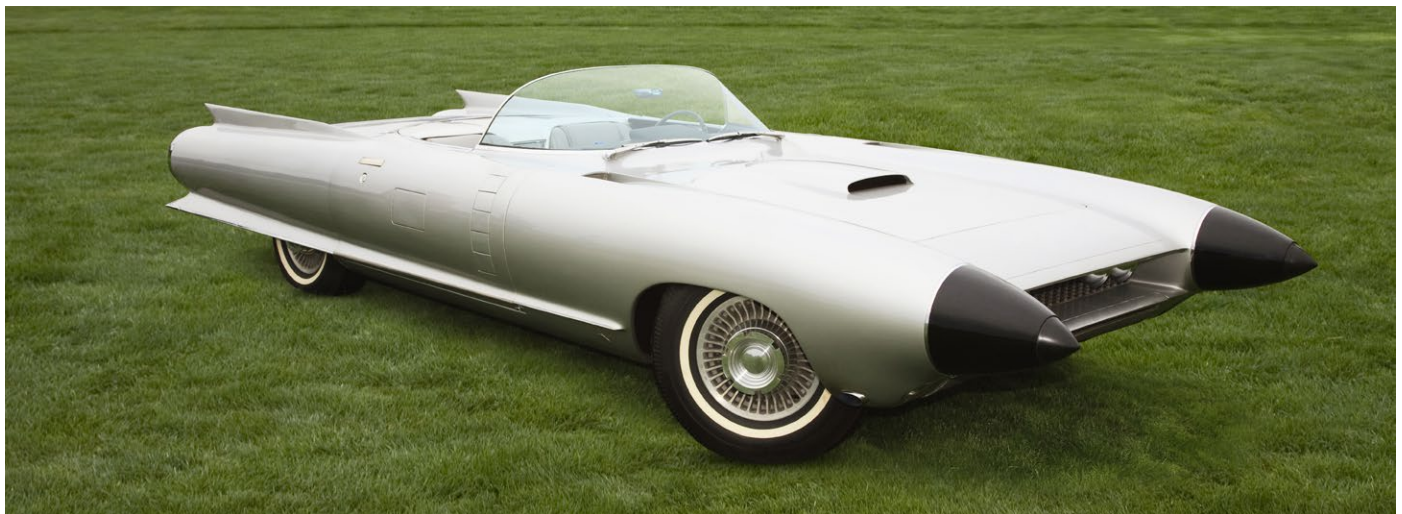
1959 Cadillac Cyclone XP-74 concept car with radar-based collision avoidance system located in the two nose cones.
